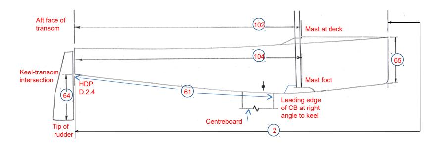
Item 2 is measured along the BL Item 61 is measured along the keel Item 102 is also shown in Deck and Interior View
